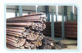
The Materials used for manufacturing bearing rings are Alloy Steel, 52100 grade and are procured from the Steel Mills approved by customers as per their specifications. We have state of the art, Metallurgical testing lab to carry out all kind of inspection of the materials received through the steel mills. To ensure the desired quality and consistency we keep track of each and every lot of steel supply received at our end. We follow system of FIFO for material usage.
